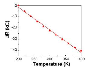
**Figure 5.** Measurements used to determine the temperature coefficient of resistance. The MWCNT change in resistance versus temperature plot is used to approximate the TCR.
